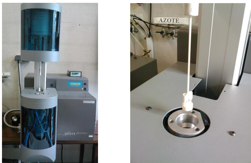
Figure 3.4: Setaram Microbalance TG-DTA92 used DTA-TGA.
