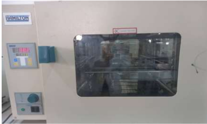
Figure (8): Drying the clove extract in a hot oven at 40 \pm 2^\circ\text{C} .
