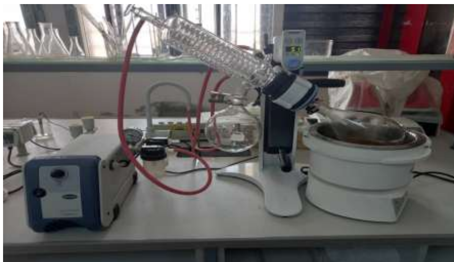
Figure (7): Separation of the clove extract from its solvent using a rotary evaporator.
