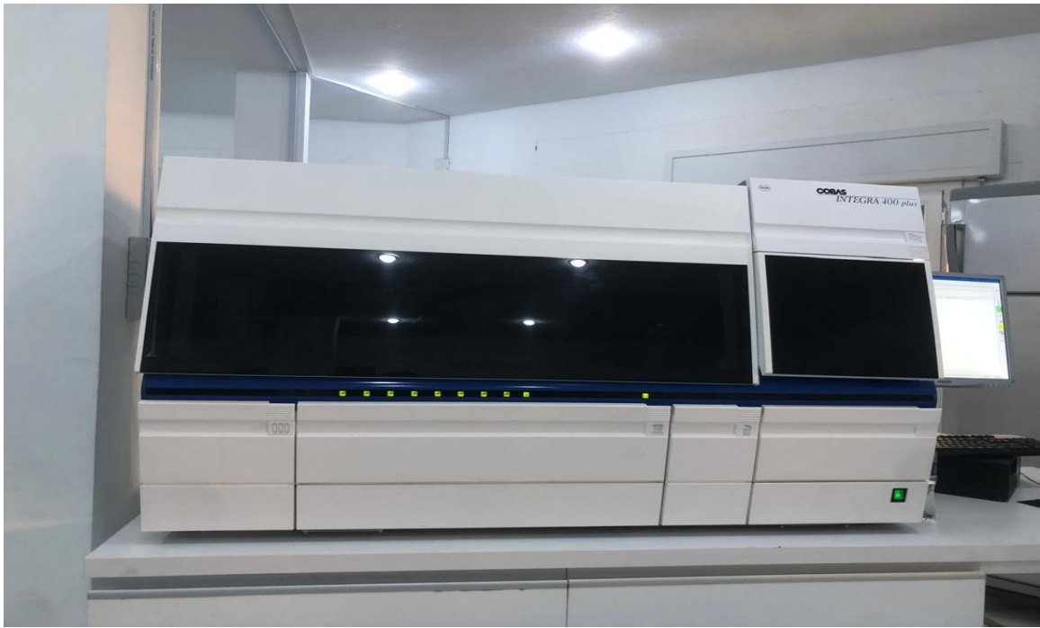
Figure 2.4. COBAS integra 400 plus used for ferritin level measurement.
