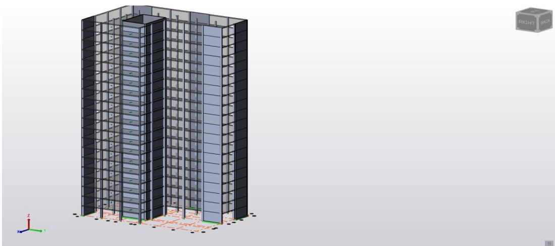
Figure 3.8 Core + perimeter walls
