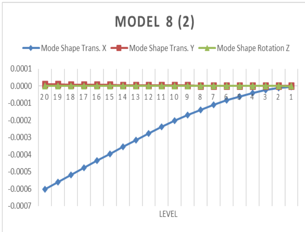
Figure 4.8 Model 8 (core + perimeter layout), Mode 2 -UX, UY, Rz versus Level
