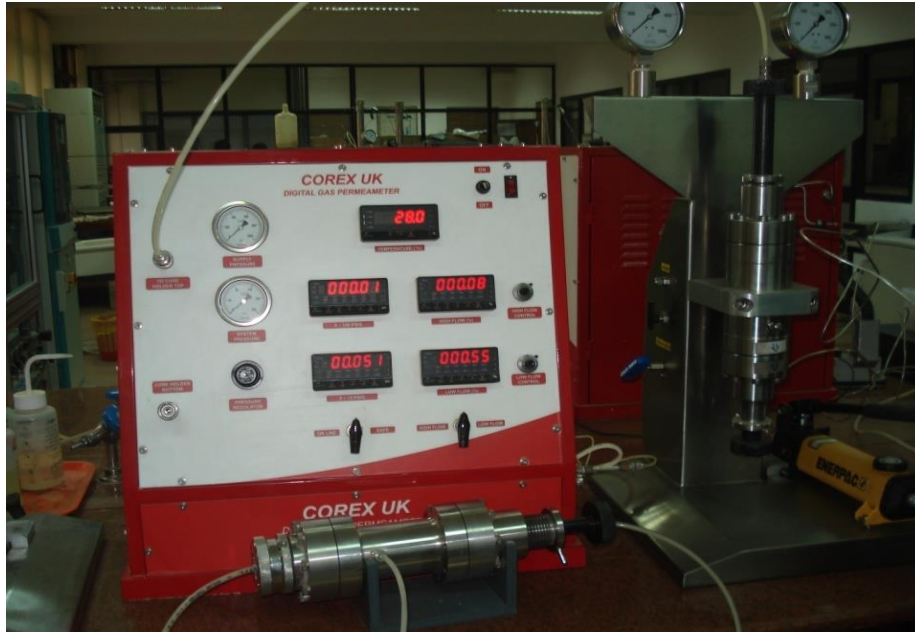
Figure (3.3): Nitrogen gas permeameter
