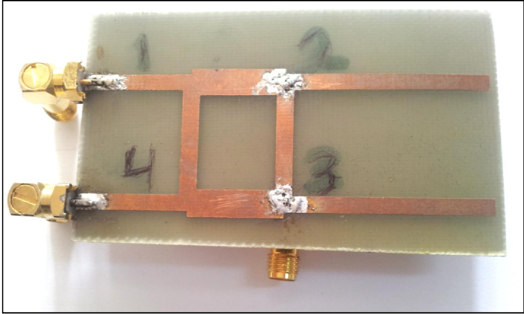
Figure (4.95) Photograph of the fabricated 90° hybrid with extended TL output ports.
