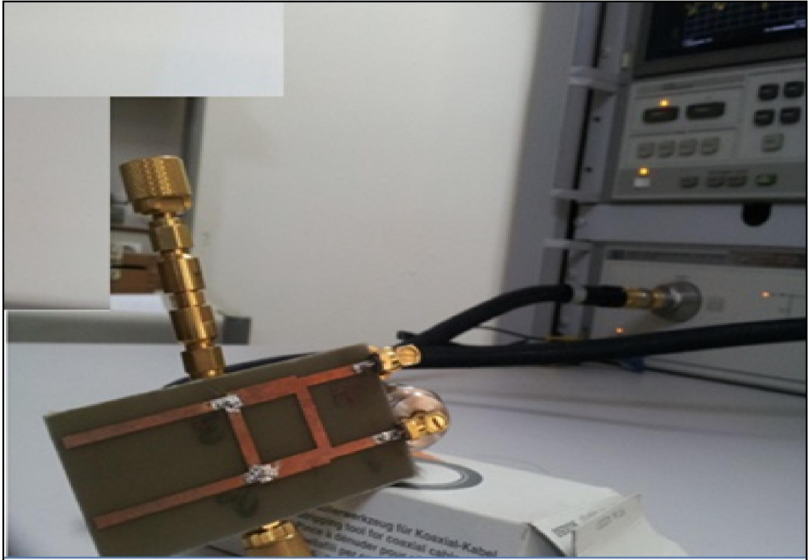
Figure (4.106) The experimental set-up of 90° hybrid with extended TL output ports.
