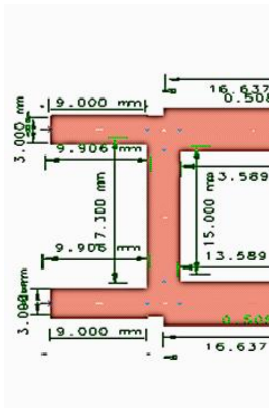
Figure (4.60) Layout of 90°hybrid with two single stub at the output ports with dimensions.
