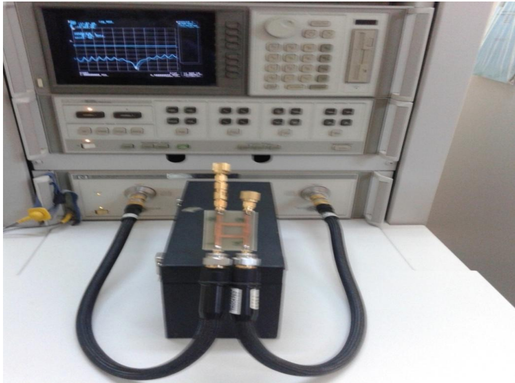
Figure (4.96) The experimental set-up of 90° hybrid measurements.
