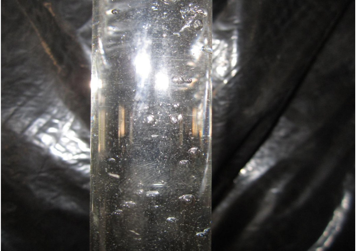
Photo (B-3) void fraction 9% Volume flow rate (24).
