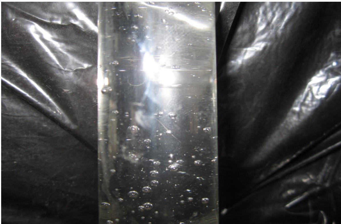
Photo (B-9) void fraction 7% at Volume flow rate (30).
