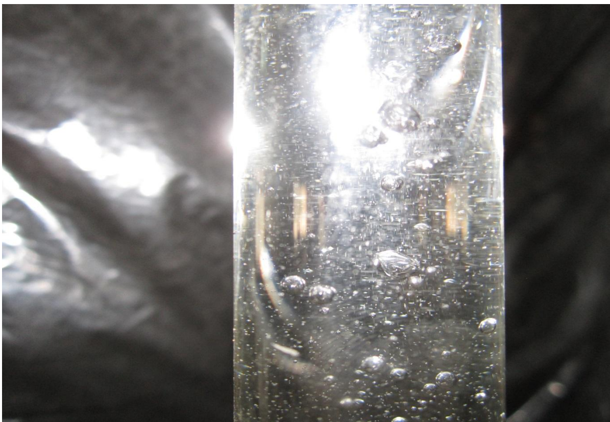
Photo (B-4) void fraction 11% Volume flow rate (24).
