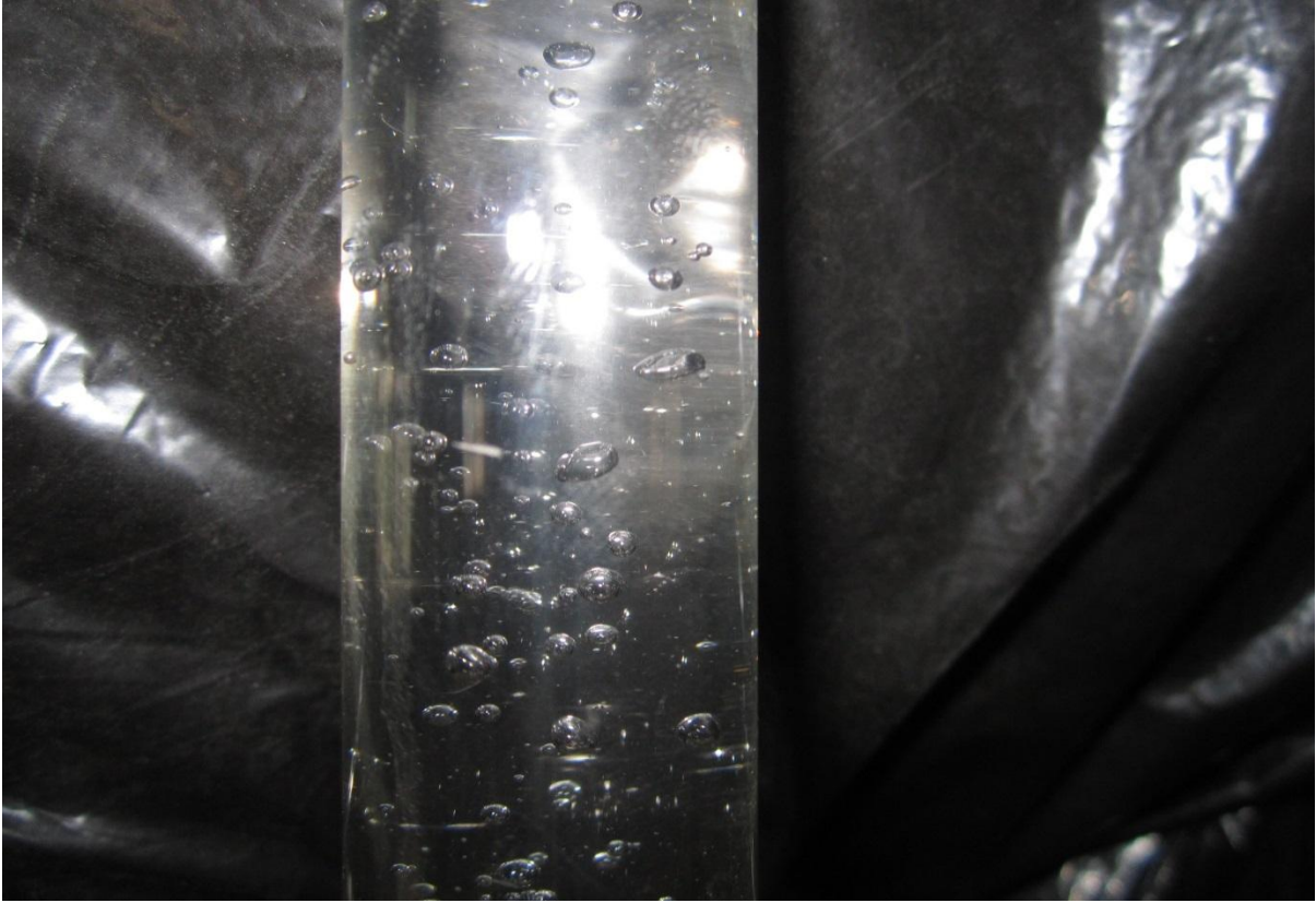
Photo (B-11) void fraction 9% at Volume flow rate (30).
