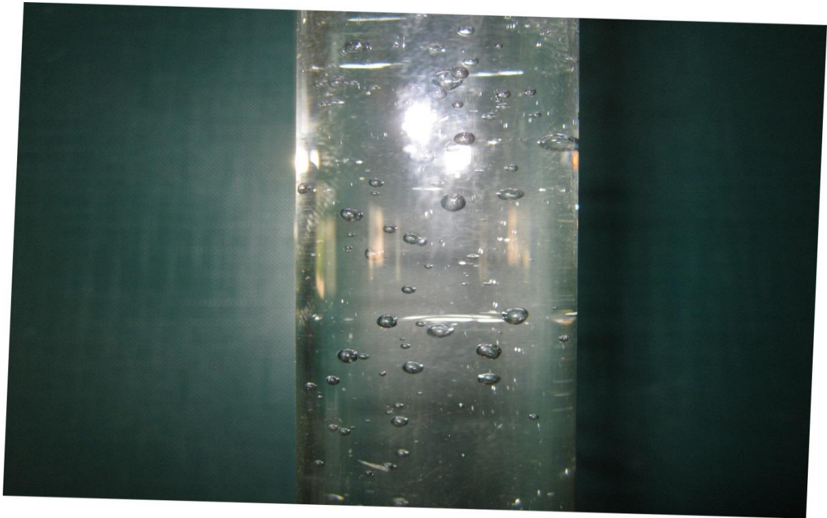
Photo (B-8) void fraction 5% at Volume flow rate (30).
