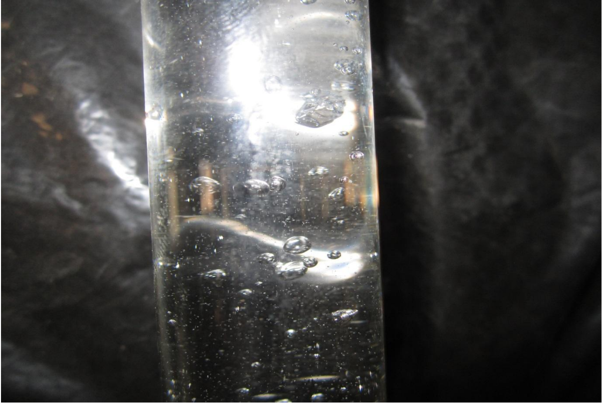
Photo (B-2) void fraction 7% Volume flow rate (24).
