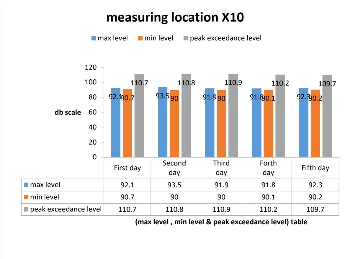
Figure 4.10 max, min and peak exceedance level at location X10, STU2.
