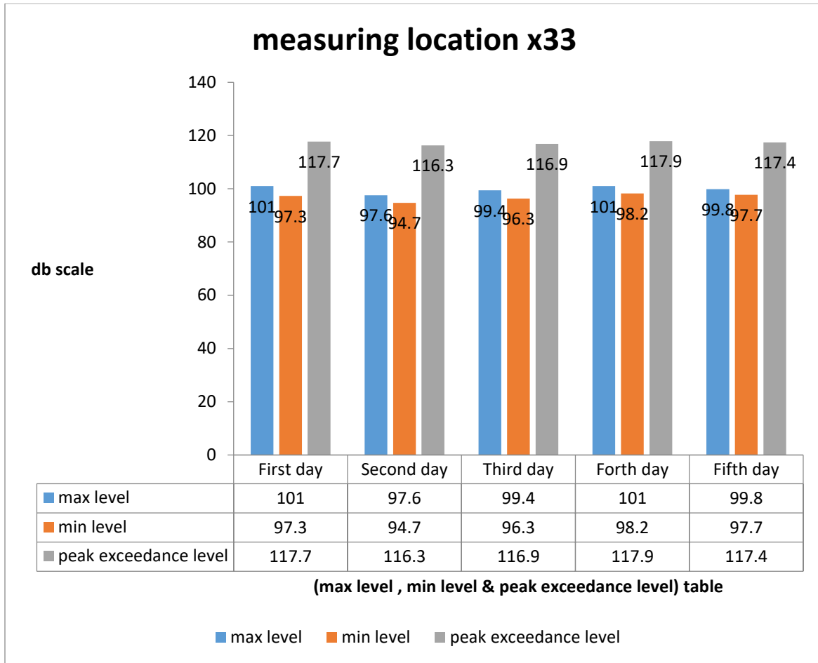
Figure 4.33 Max, min and peak exceedance level at location X33, GTU14.
