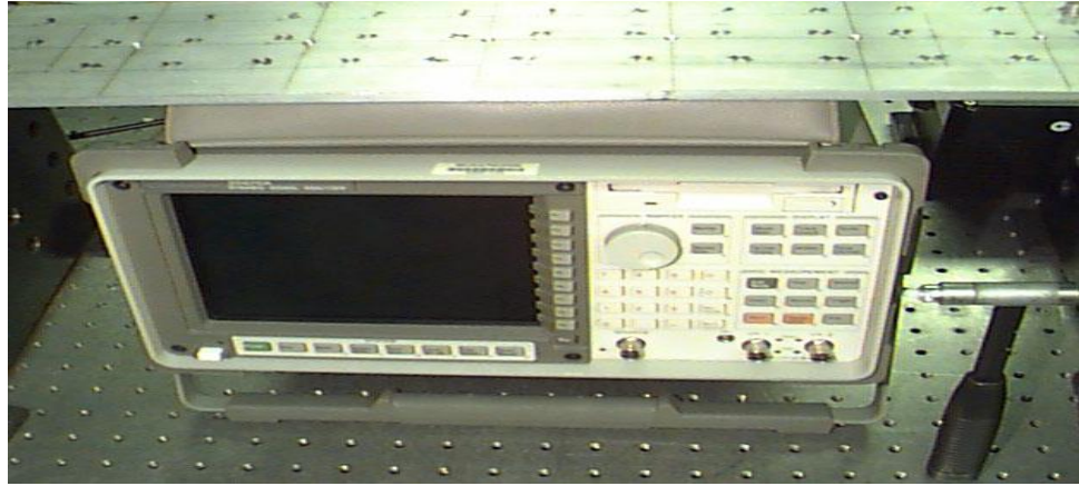
Figure 2.18 Portable 2-channel acoustics and vibration data acquisition system. [34]
