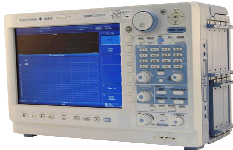
Figure 2.13 The Yokogawa DL850 ScopeCorder 100 MS/s, 8 slots. [29]
