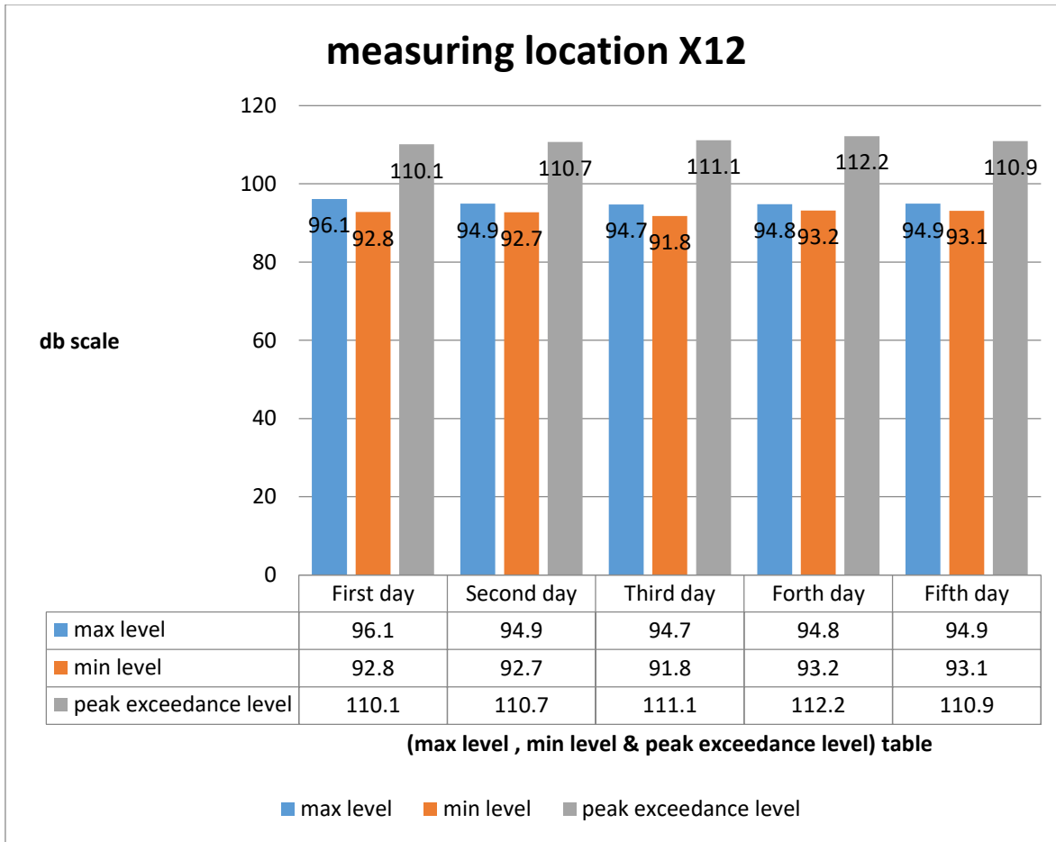
Figure 4.12 Max, min and peak exceedance level at location X12, STU2.
