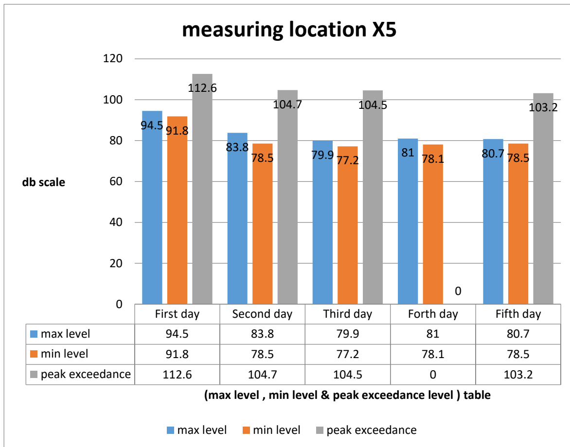
Figure 4.5 Max, min and peak exceedance at location X5, STU3.
