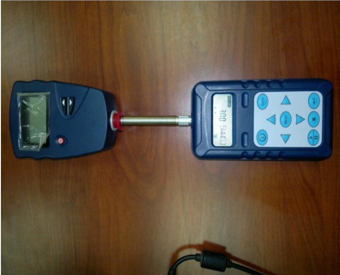
Figure 3.36 Calibration to sound level meter device by calibrator device
