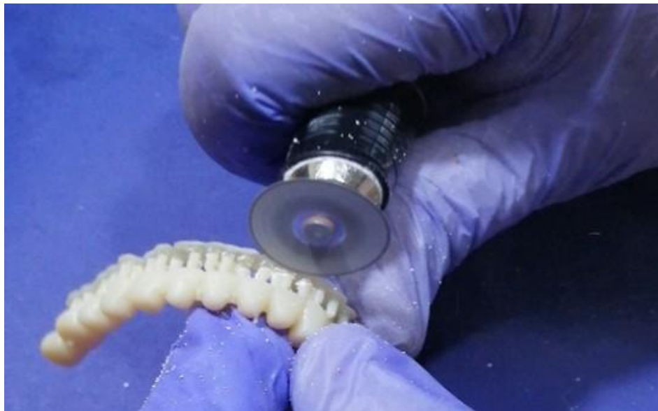
Fig. (18): Removal of supporting structures
