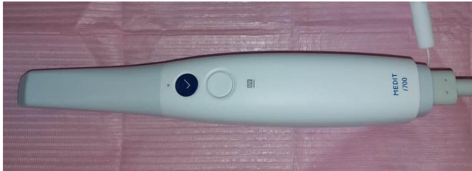
Fig. (28): Medit I700 intra-oral scanner
