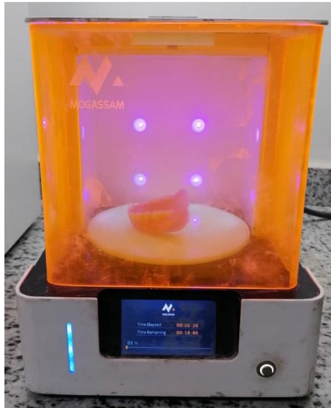
Fig. (19): Denture base was bonded to dental arch by the aid of light curing unit
