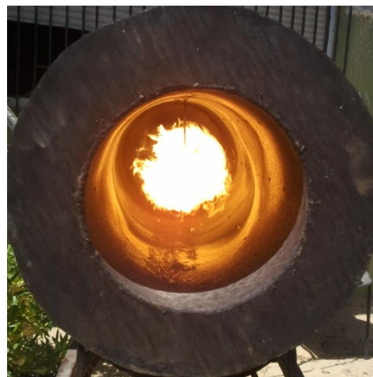
Photo. (4.3) With primary air and secondary swirl (Case B)
