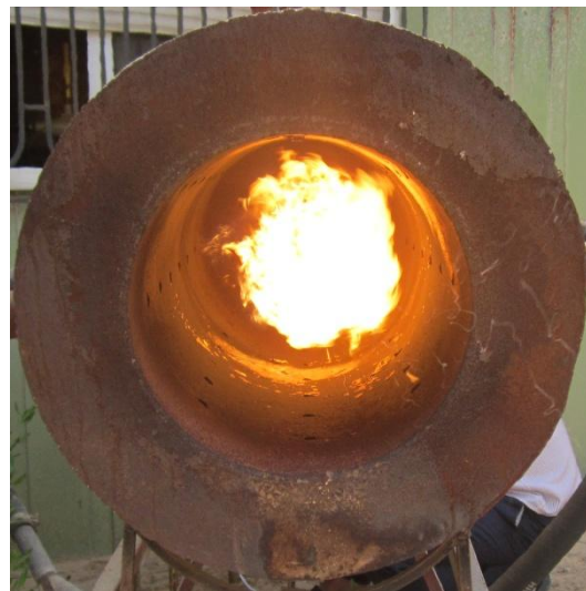
Photo. (4.2) With primary air and secondary swirl (Case A)
