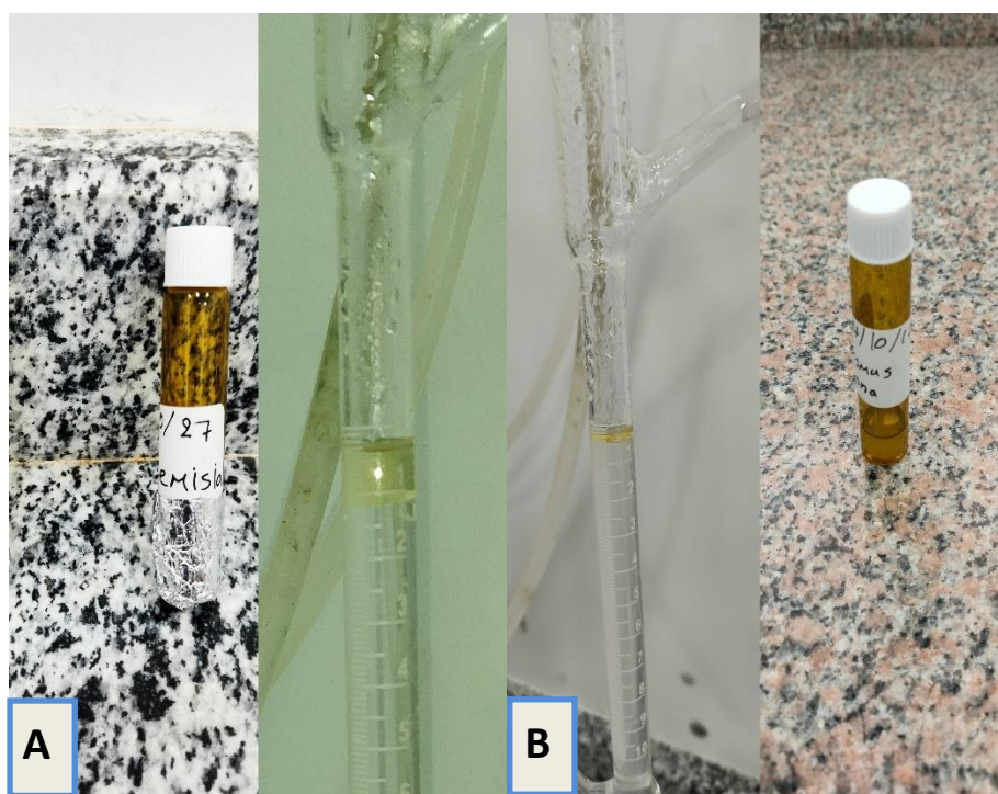
Figure (3-1) Extract of (A) A. herba alba and (B) T. capitatus essential oil by hydro-distillation using a Clevenger apparatus.
