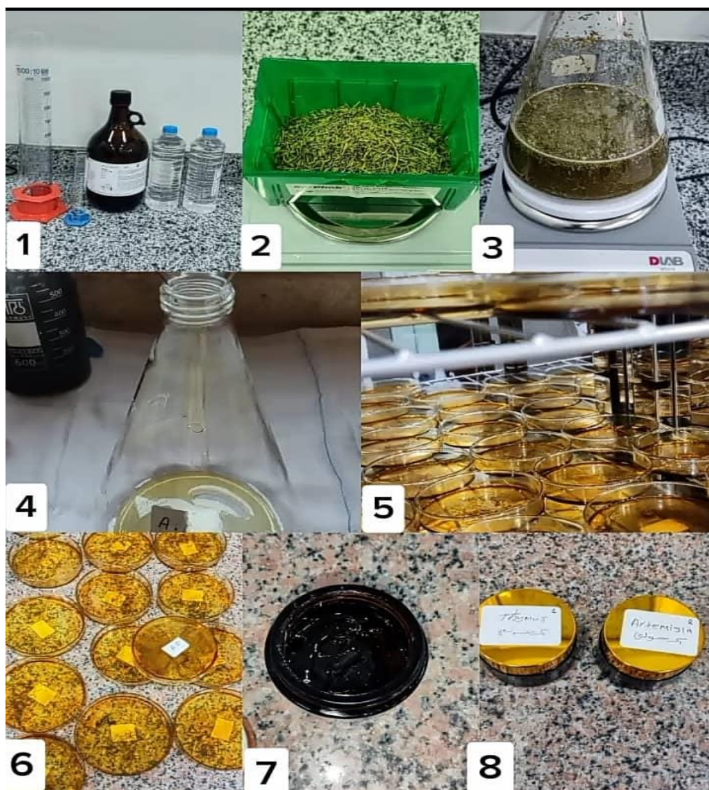
Figure (2-4) Show the steps for preparation of alcoholic extract.
