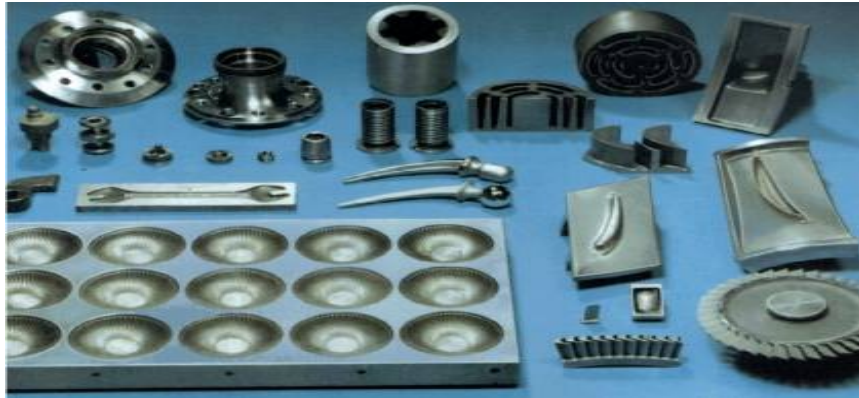
Figure 3.11 Parts made by ECM
