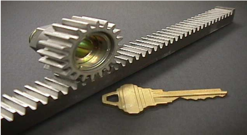
Fig(3.19) Steel gear and rack cut with an abrasive water jet
