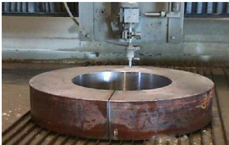
Fig(3.18) Abrasive water jet cutting
